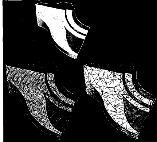
Figure 19: Preserving feature-lines. The original fandisk model (top and bottom-left) of 12,946 faces is simplified to 1,632 faces (bottom-right). The feature-lines are red.
