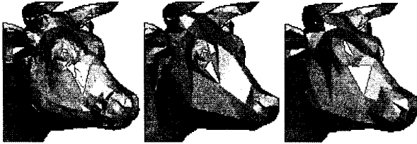
Figure 10: Comparison with QEM. The original model of 5,804 faces (left), and simplified models of 2,000 faces using our scheme (middle) and QEM (right).
