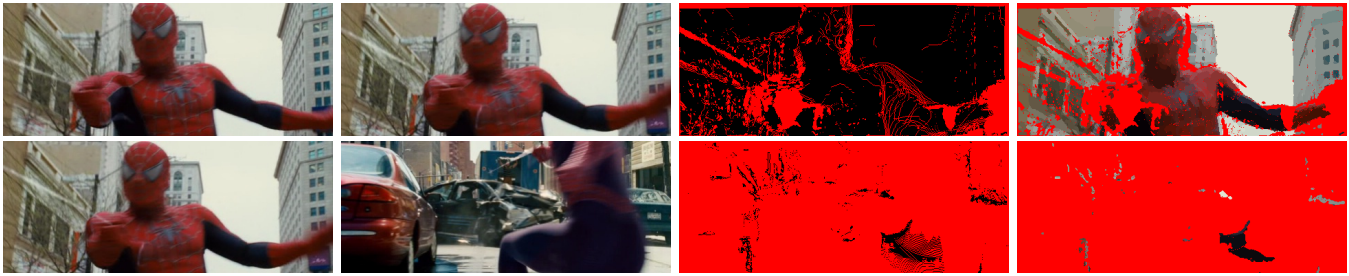
Fig. 8. Label propagation by optical flow: 2 examples. From left to right: previous frame, current frame, residual map before morphological filtering, propagation map after morphological filtering.
