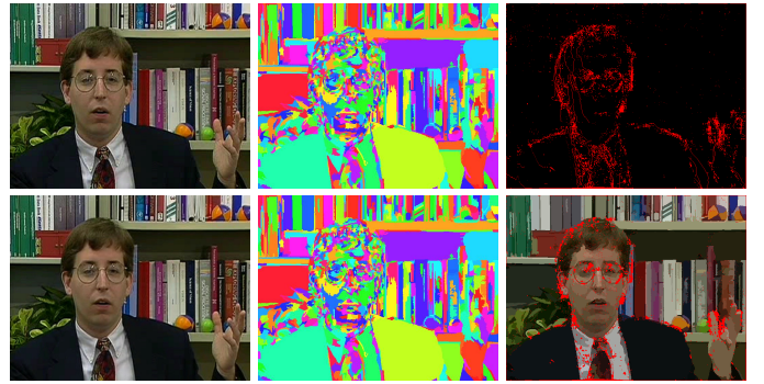
Fig. 3. Left: input frames 1, 2. Middle: segmentation results for frames 1, 2. Right-top: residual map before morphological filter. Right-bottom: region label propagation result after morphological filter.
