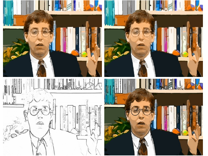
Fig. 5. Boundary smoothing and edge overlaying. Top-left: segmentation result. Top-right: after boundary smoothing. Bottom-left: detected lines. Bottom-right: smoothed result after edge overlay.
