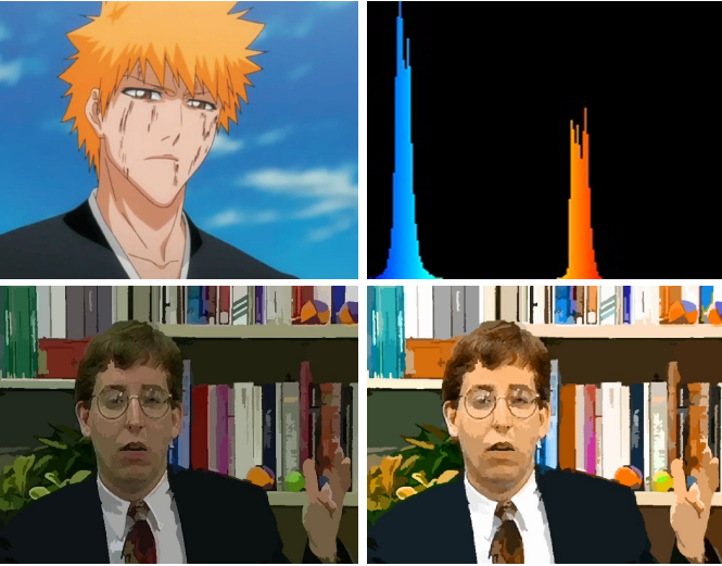
Fig. 4. Color scheme replacement. Top-left: a frame of the reference video. Top-right: histogram of its H channel. Bottom-left: segmented frame before replacement. Bottom-right: frame after replacement.
