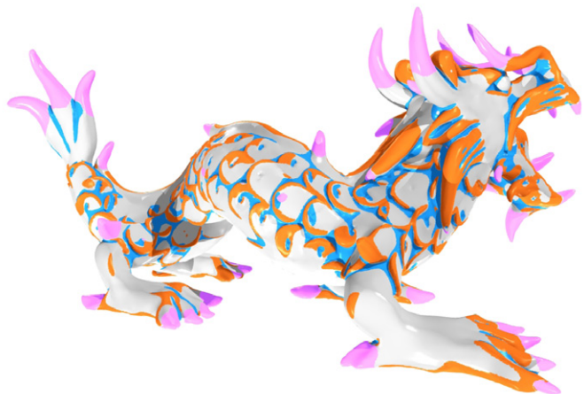
Fig. 1. Result of automatic feature classification: ridges (orange), valleys (blue), prongs (pink). See also Fig. 10.
