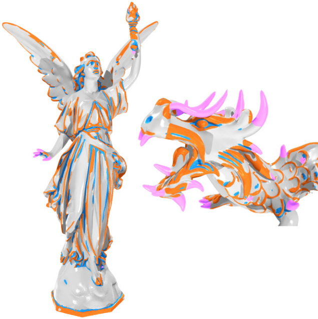
Fig. 10. Automatic detection and classification of features: ridges (orange), valleys (blue), prongs (pink). cf. Fig. 1.
