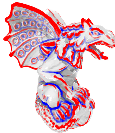
Figure 1: Feature extraction on multiple scales using PCA on ball neighborhoods of different radii. Darker regions are classified as features on all scales, lighter shaded regions correspond to features extracted at only one or two scales.
