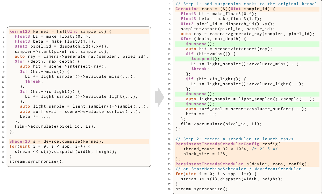
Fig. 3. A typical use case of rewriting a mega-kernel path tracer (left) using GPU coroutines and scheduling it with the built-in scheduler (right). Step 1: Users can conveniently specify the splitting points using the $suspend keyword, and the system automatically handles the code transformation and live state computation. Step 2: Multiple built-in schedulers, such as the persistent-threads model, are available for scheduling the execution and managing the states of massively parallel coroutine instances on the GPU device.
