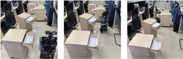
Fig. 7. Snapshots of real robot navigation with our novel DRL framework. Note that the drawers at high positions serve as obstacles that do not exist near the ground.
