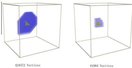
Fig. 8. The dependent set (blue voxels) for synthesizing a triangular object,  $N = 5, P = 3, s^3 = 8$ , normal correction (left), and dual-grid correction (right).
