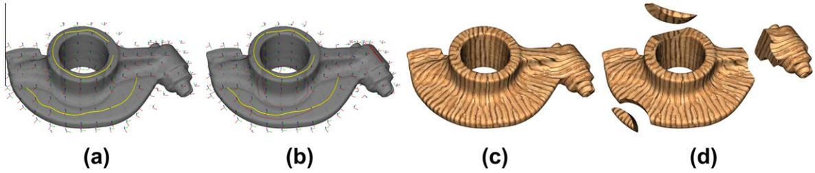
**Fig. 3.** Sketch guided 3D tensor field generation. Smooth tensor fields are interactively obtained while users adding sketches (a and b). Solid textures are consistently produced w.r.t. the field on the bounding surface (c) or in the interior on demand (d).
