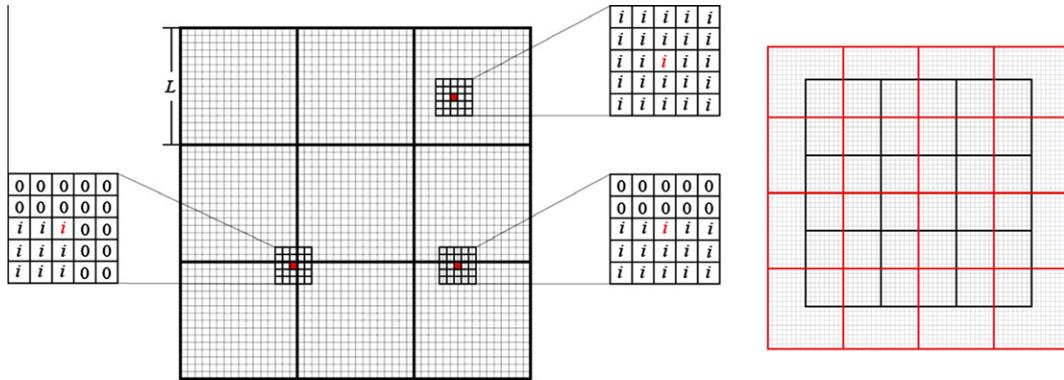
Fig. 7. Left: grid correction with related history windows. Right: dual grid arrangement in red following primary grid in black for improved continuity.
