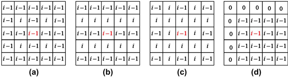
Fig. 6. History windows for different correction schemes. (a–c) history windows used in 2nd, 3rd and 4th subpasses for  $s^2 = 4$ ; (d) a constrained scheme using version 0 to stop the growth of the dependent set.
