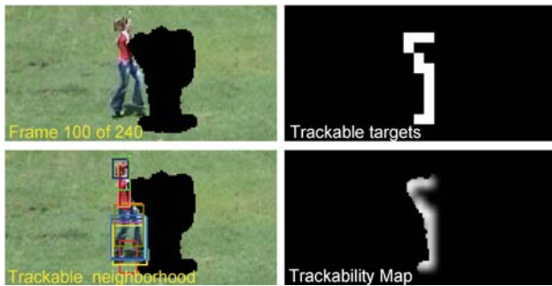
Fig. 4. Top left to bottom right: source frame, trackable target fragments, trackable neighborhoods of target fragments, trackability map of source frame
