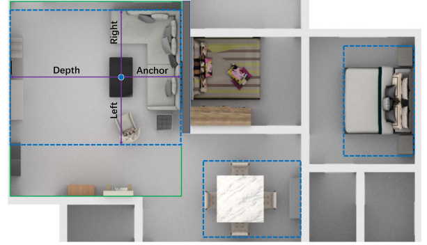
Fig. 6. Illustration of derived spaces. A derived space (blue dotted lines) of a coherent group G_i is defined by the anchor, left, right, and depth (purple arrows) w.r.t the dominant object (blue circle). The distance between the nearest boundary to the dominant object creates the anchor. A derived space (green solid lines) of \vec{x} and R is conducted by further expanding D(G_i) so that a larger square is fitted to the room shape.
