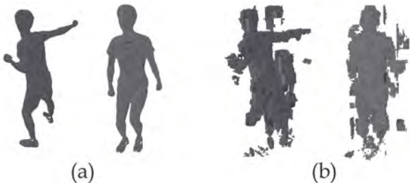
Fig. 9: Comparison with OGN. (a): Occupancy maps reconstructed by 3D-CFCN. (b): Occupancy maps decoded by OGN, using features learned by 3D-CFCN.
