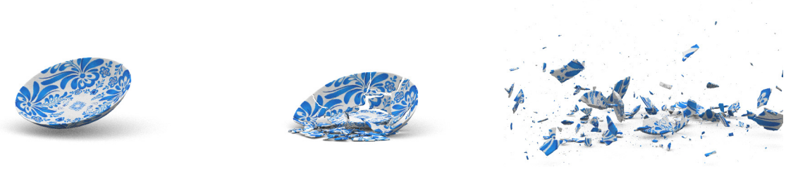
Fig. 3. A ceramic plate dropped on a hard floor and broken into pieces. Our simulation captures highly detailed fractures using only 219K particles, with a 2.4x speedup over the state-of-the-art method.
