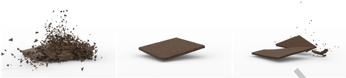
Fig. 8. This figure, from left to right, demonstrates the fracture performance of FEM, MPM, and our method under the high-speed drop impact of a chocolate object. The FEM resulted in an excessive fragmentation into minute pieces, while the MPM failed to produce a physically plausible fragmentation. In contrast, BDEM accurately fragmented into a variety of piece sizes, effectively capturing the desired material failure behavior.
