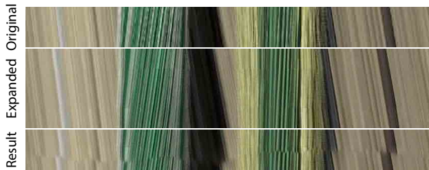
Figure 18: Here, the original light field (100 views) is expanded to 200 views using image-based warping. After stitching, the resulting light field has the same number of views as the input content. Please refer to the supplementary materials for the complete light field.
