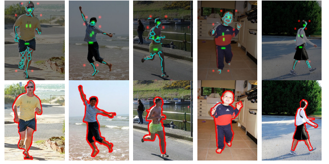
Fig. 4. Character segmentation results. The first row shows the automatically identified ‘definite human pixels’ (green) and ‘definite background pixels’ (red). The second row are results from graph-cut based segmentation.
