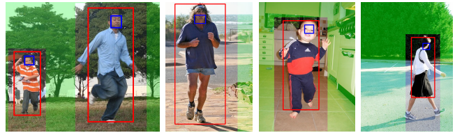
Fig. 2. Human detection results. The red frame is the bounding boxes of detected human. The blue frame indicates detected faces. The region overlaid in green contains ‘definite background pixels’.
