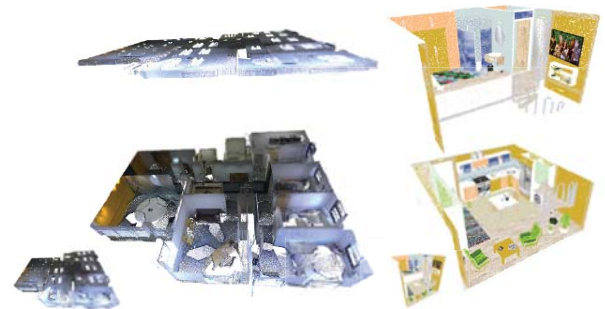
Fig. 3 Decomposition of one-storey (left) and two-storey (right) buildings into individual storeys, with the removal of ceilings (if any).
