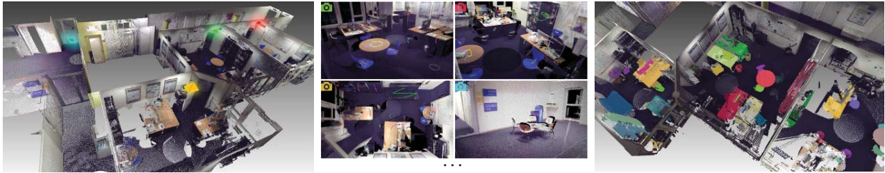
Fig. 1 Given an input scene represented as a 3D point cloud (left), our system automatically suggests a series of reasonable views (middle) for easily inputting segmentation hints for semantic segmentation of the entire scene (right).
