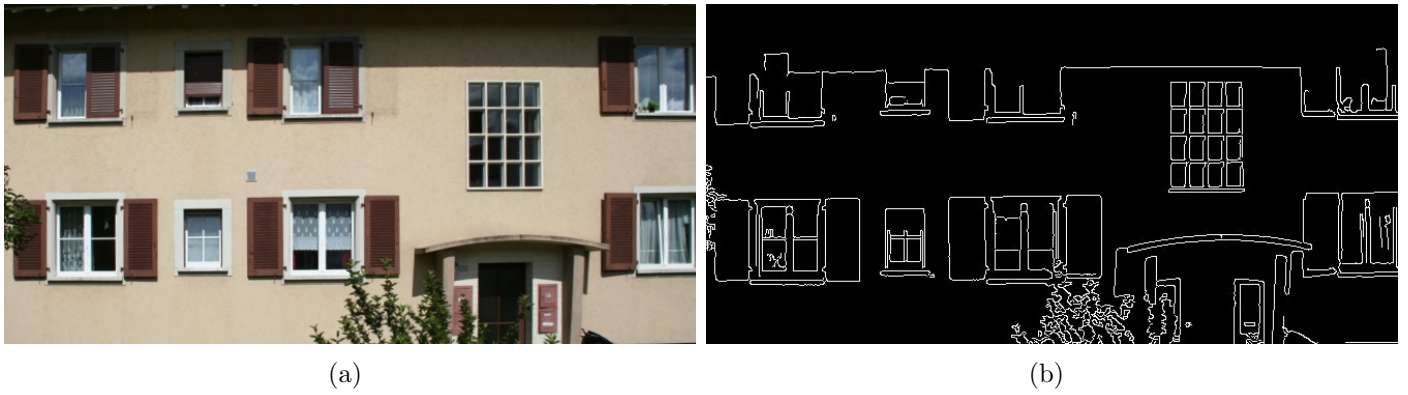
Figure 1: Input image and detected edges
