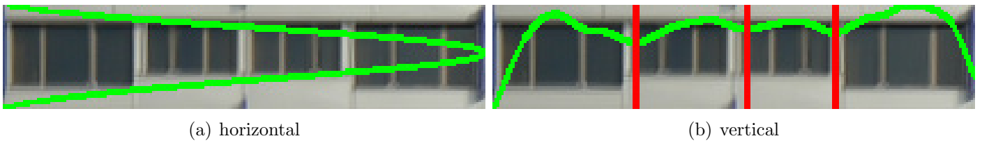
Figure 6: Level 2, group 2, penalty function. Determined splitting direction: vertical.
