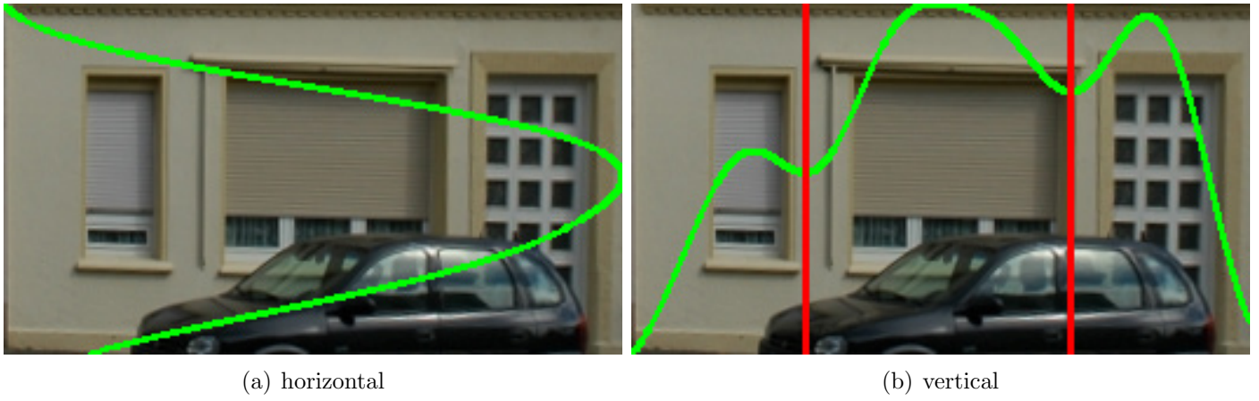
Figure 8: Level 2, group 3, penalty function. Determined splitting direction: vertical.
