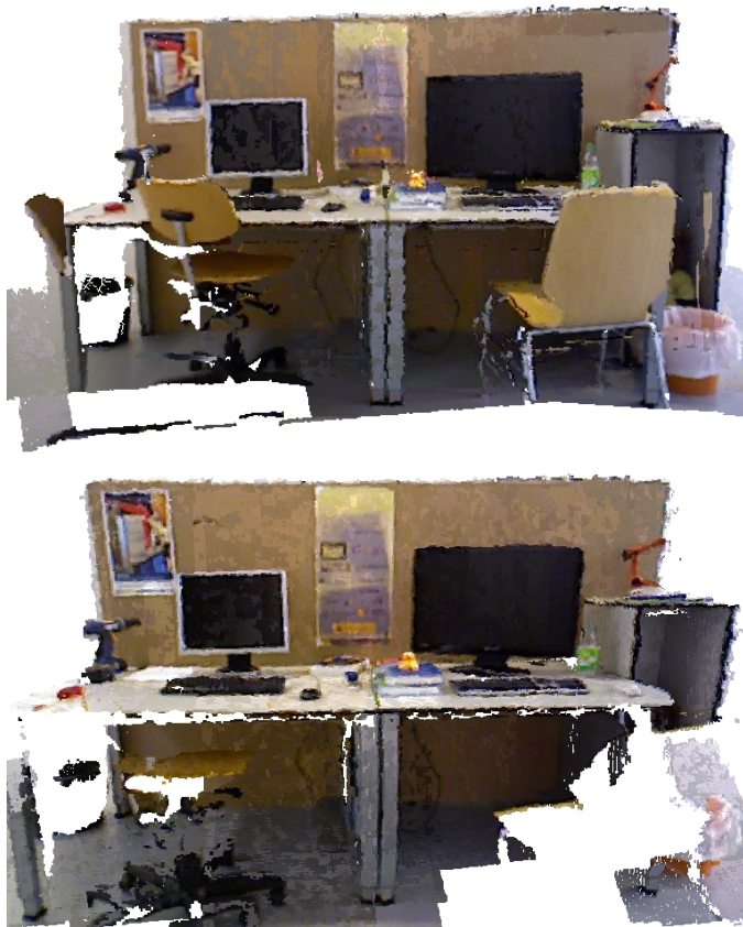
Fig. 9. The reconstructed point clouds for two scenes (top: fr3/walking-xyz, bottom: fr3/walking-static) from TUM RGB-D dataset.
