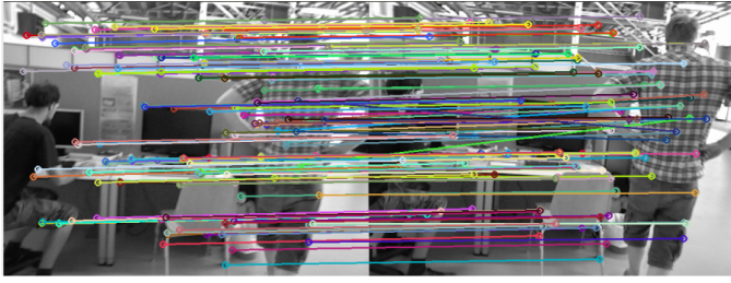
(a) Feature matching between reference frame and current frame before GC-RANSAC
