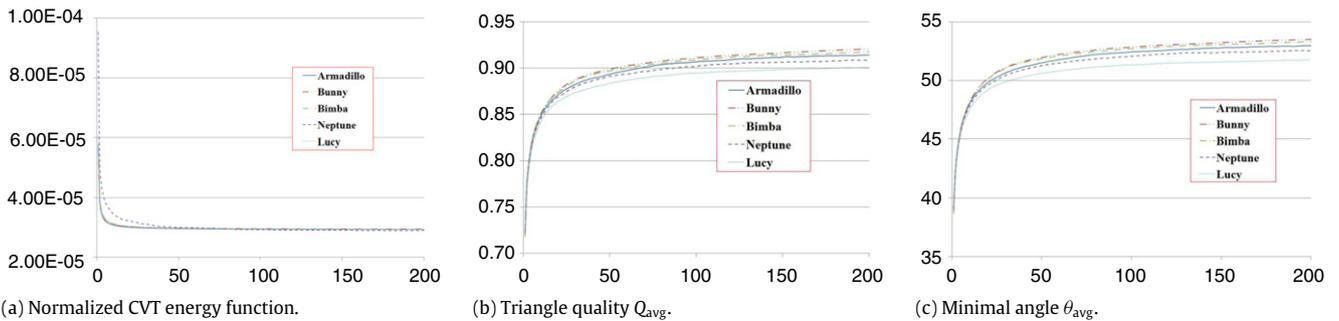
Fig. 10. Energy function and quality measures. The horizontal axis in the plots shows the iteration number. The vertical axis in (a) is the *normalized CVT energy function*, that is,  $\frac{F(S)}{A^2}$ , where  $A$  is the area of the model.
