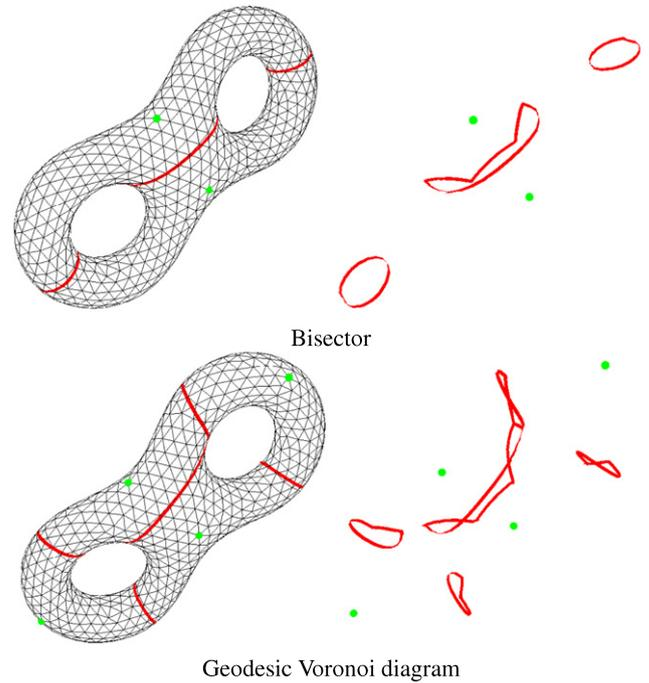
**Fig. 3.** Bisector and geodesic Voronoi diagram. Row 1: The bisector (red) of two sites (green) on the double-torus has three separated components. Besides line segments, a bisector on triangle mesh may also contain hyperbola segments. Row 2: The geodesic Voronoi diagram of four sites. Each Voronoi cell is bounded by two or three closed bisectors. (For interpretation of the references to colour in this figure legend, the reader is referred to the web version of this article.)
