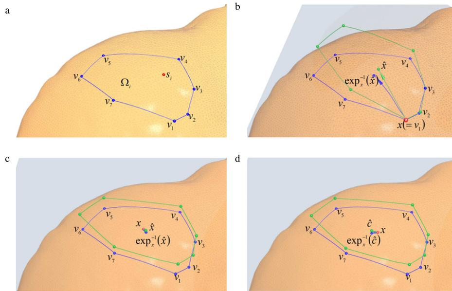
**Fig. 6.** Computing the center of mass for the Voronoi cell  $\Omega_i$ . It takes two iterations (b) and (c) to obtain the Riemannian center  $c$ . The blue dot  $\exp_x^{-1}(\hat{c})$  in (d) is the center of mass. (For interpretation of the references to colour in this figure legend, the reader is referred to the web version of this article.)
