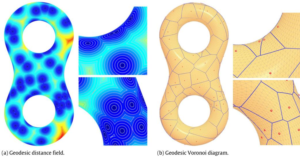
**Fig. 5.** The multiple-source geodesic distance field induces a geodesic Voronoi diagram. The cold (resp. warm) color in (a) indicates the small (resp. large) geodesic distance. (For interpretation of the references to colour in this figure legend, the reader is referred to the web version of this article.)
