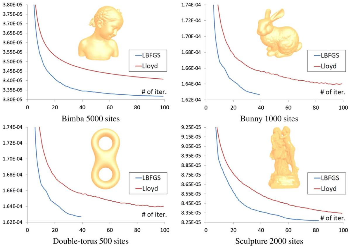
Fig. 7. Convergence rate comparison between the Lloyd method and the L-BFGS method.
