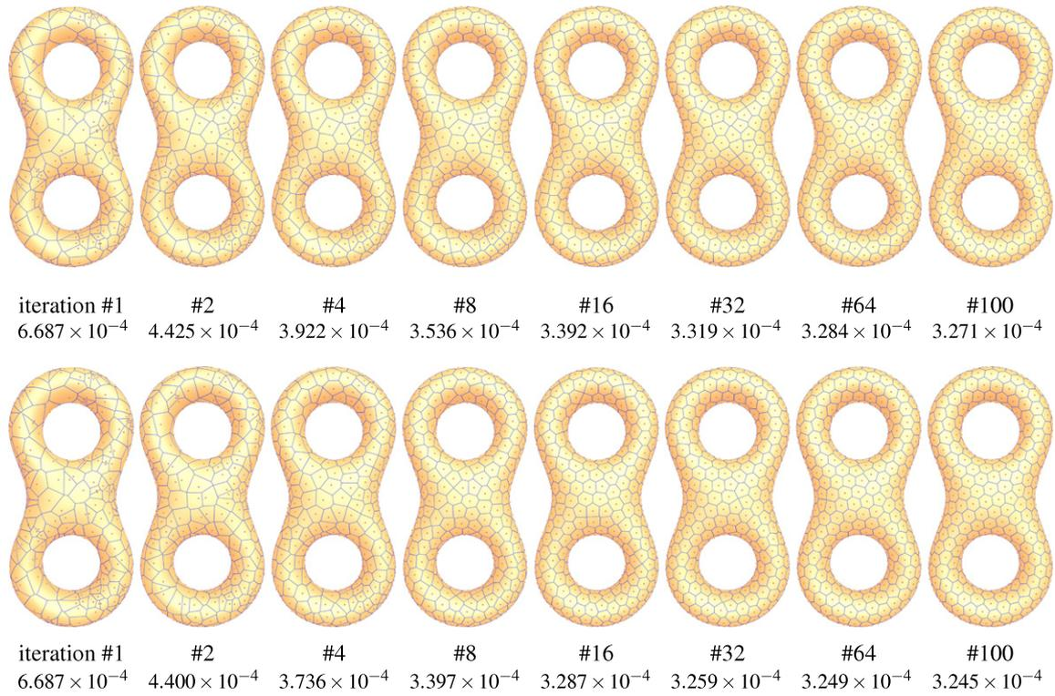
Fig. 4. Iteratively computing geodesic CVT on meshes. Row 1: the Lloyd algorithm; Row 2: the L-BFGS algorithm.
