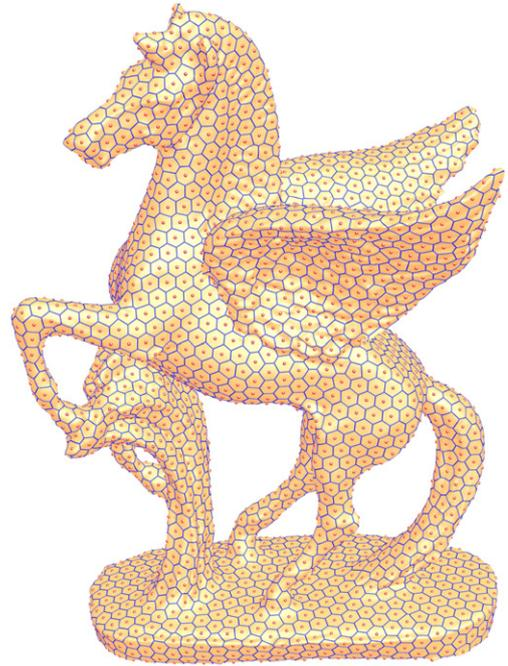
Fig. 1. Our intrinsic method can compute a high-quality centroidal Voronoi tessellation on model with complicated geometry and topology. The CVT on the Pegaso model was created by 3000 sites.
