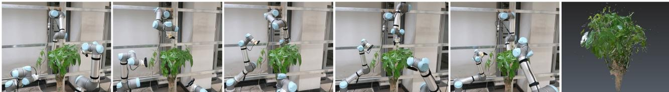
Fig. 5. The progressive views of plant phenotyping by our multi-robot. These pictures are taken when our multi-arm system is running the proposed deep NBV planner. The last column depicts the resultant point cloud of the plant. One can watch the accompanying video for a full illustration.
