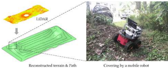
Fig. 10. Experiments taken in an outdoor environment for verifying the energy consumption by following a zig-zag path vs. a spiral path generated by our method (see the path shown on the reconstructed surface).
